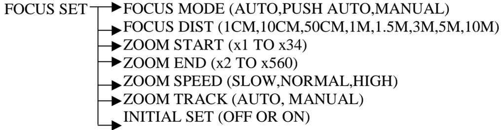
**FOCUS MODE** Set up of automatic focus option. This allows the user to control the adjustment of the focus automatically by the module (AUTO) or when set to (PUSH AUTO) the camera module will do a single push to focus the camera and will not try to refocus after the initial push or to allow the operator to adjust the focus manually using the NEAR & FAR buttons on the keypad (MANUAL).
