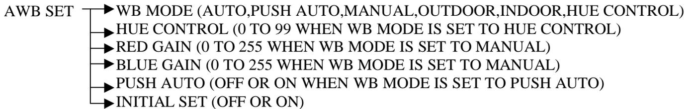
**WB MODE**                      This option is used to instruct the module of the environment in which it is installed and which mode to use to adjust the white balance of the image output. The options are AUTO, PUSH AUTO, MANUAL, INDOOR, OUTDOOR or HUE CONTROL.
